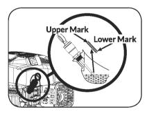
3. Using a funnel, add oil up to the FULL mark on the dipstick. (See engine manual for oil capacity, oil recommendation, and location of fill cap.)
