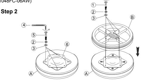
Attach the swivel to the seat and the frame. Please note that long holes on the sviwel go toward the seat and the holes with inserts go away from the seat.
