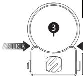
NOTE: Ring clamps 2" & over in size may require pre-stretching to help spread the clamp over the tube. (Use Protective film when mounting)
