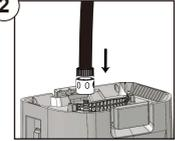
Pull back the adaptor collar and attach to the male connector on the machine.
