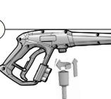
Push and turn clockwise one end of the high pressure hose into the inlet coupler.
