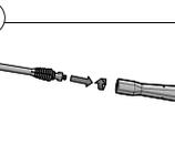
Assemble pressure washer gun to spray wand.
