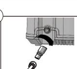
Thread the priming valve onto the pressure washer outlet and rotate clockwise until tightened. Once installed, take the end of the included high pressure hose and tighten onto the valve.
