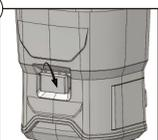
Lift and push down the bucket buckle to fix the bucket.
