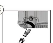
Place the valve onto the pressure washer outlet and rotate clockwise until tightened. Once installed, take the end of the included high pressure hose and tighten onto the valve.
