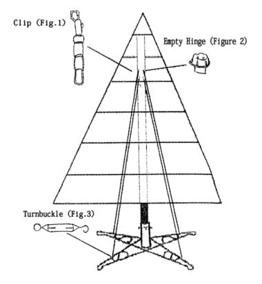
**WARNING:** Please do not attempt to straighten the tree with the stand bolts. The cables are the mechanism to straighten the tree.
