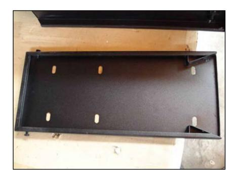
3. Position the mounting tray behind the fender flare of your choice, ensuring to have the front facing the tailgate.
