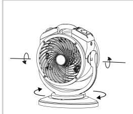
• The misting fan can operate in different positions, directing the airflow and mist to desired areas.
