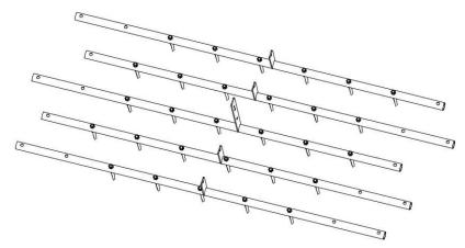
2. Insert Lift connecting plate (#6) and Right connecting plate (#7) into the Pipes (#1#2#3) in turns.
