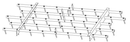
4. Attach connecting board on the pipes and Connect flat bar (#9) with Self-locking nuts (#11) and Bolt (#12). Install Regulating flat bar (#8) on the last hole. Attach Regulating flat bar (#8) and middle pipes with Bolt (#12), Spring washer (#14), Washer (#15) and Bolt (#16).
