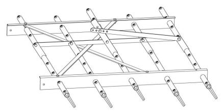
Attached Long chain (#17) and Short (#18) to Lift connecting plates (#6), Right connecting plate (#7) and 3pt connector (#4) with Self-locking nuts (#11) and Bolt (#12). Insert Pin (#19) into 3pt connector (#4).
