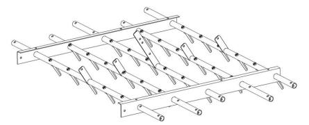
3. Install remaining 16pcs Spikes (#5) on the Pipes (#1#2#3) with Self-locking nuts (#13) as below picture shows. Note: All the Spikes are facing same direction.
