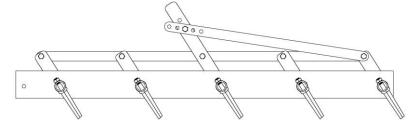
5. Attach Fixed flat bar (#10) and two Lift connecting plates (#6) and Right connecting plate (#7) with Self-locking nuts (#11) and Bolt (#12).
