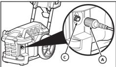
NOTICE DO NOT siphon standing water for the water supply. Use ONLY cold water (less than 90°F (32°C)).
