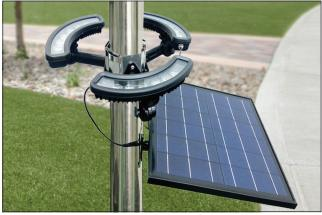
Our 1980 lumen solar flag pole light is a set of three light heads, each containing 6 bright LEDs covers 360 degree angle. Each head can be individually adjusted to beam at different directions using 180 degree know adjustment. Solar panel is glass protected and the light heads are made from die cast aluminum. The light is designed to come on/off automatically from dusk to dawn.
