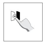
**Reminder:**The remaining time of filter life is more than 432 hours, and the filter life progress light is always white. The remaining time of filter life is less than 432 hours, and the filter life progress light turns red and stays on. When the remaining time of filter life is zero, the filter life progress light flashes red, and the indicator light flashes when replacing the filter life.
