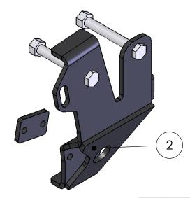
SOME FRAMES MAY ONLY USE FRONT BOLT HOLE AND NOT REQUIRE OR ALLOW INSIDE FRAME PLATE TO BE USED
