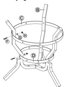
**NOTE:** Posts (A and B) install on the inside of rings (C and D). Leg Posts (B) must be evenly spaced, with 2 mounting holes between each leg, as shown.
