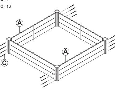
Align remaining two Side Panels (A) between the corner posts of the assembled components.
