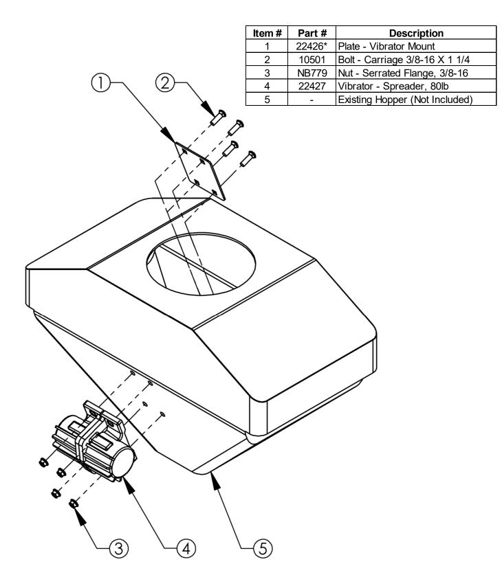
Spreader Vibrator shown on a Swisher ATV Spreader.
