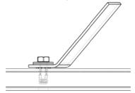
8) Place (2) of the isolation bumpers on top of the rail aligned with the jack nut and the mounting hole on the UTV Cargo Box /Cooler Combo Box.
