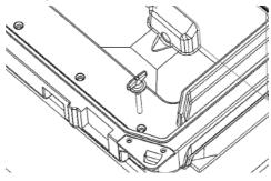
10) Place the plastic plugs (included) into the mounting holes that were not used to seal the box and keep out contaminants.
