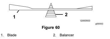
3. Repeat this procedure until the blade is balanced.
