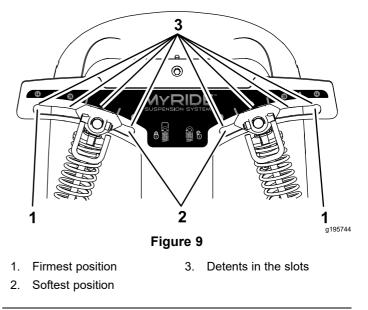
**Note:** Ensure that the left and right springs are always adjusted to the same positions.
