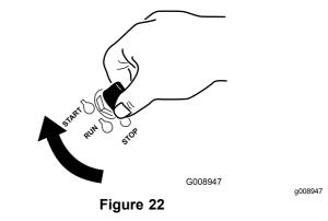
2. Turn the key to the STOP position to shut off the engine.
