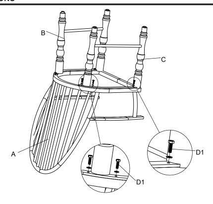
Do not tighten completely. Repeat procedure for the other side. Securely tighten all bolts.
