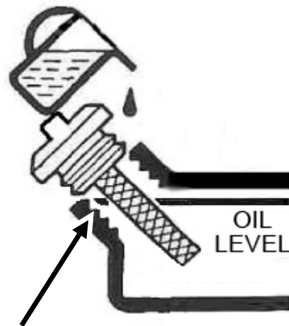
Figure 2 - Add Oil To TOP Of Threads
