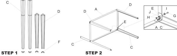
Slide the Plastic Feet (F) onto the ends of the legs (C & D).
