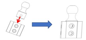
a. Align the hitch ball hole with the center of the bracket hole
