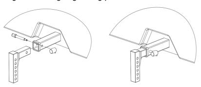
Step 2: Install hitch ball(s) to adjustable section. See pin assembly below. Note: You can tow with one or both hitch balls installed.
