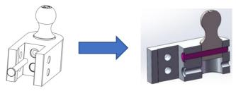
Step 3: After installing hitch balls to adjustable section. Slide the adjustable section onto the aluminum drop at desired height and secure with the locking hitch pin and standard hitch pin. ALWAYS use both pins to secure adjustable section to the drop.
