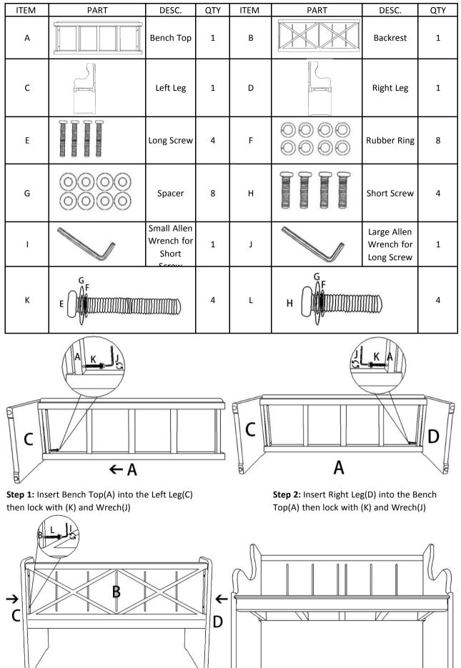
**Step 3:** Insert Backrest(B) into the Bench Top(A) and Leg(C,D) then lock with (L) and Wrench (I)
