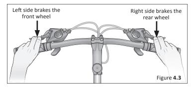
to check how your bike's brakes are set up, squeeze one brake lever and look to see which brake, front or rear, engages. Now do the same with the other brake lever.
