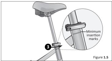
If your bike has an interrupted seat tube, as is the case on some suspension bikes, you must also make sure that the seat post is far enough into the frame so that you can touch it through the bottom of the interrupted seat tube with the tip of your finger without inserting your finger beyond its first knuckle. Also see NOTE on previous page.
