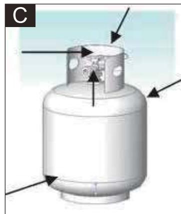
5. Slowly turn the LP cylinder valve counterclockwise to the open position.
