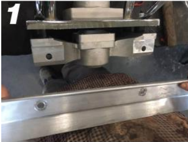
Line up blade with assembly.
