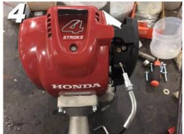
Connect accelerator cable to engine.
