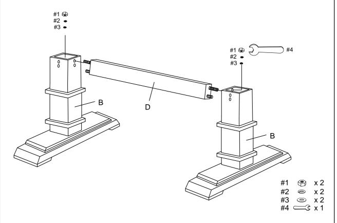
Step 2 . Attach bench supports (part E) to legs (part B) using flat washers (part #3), spring washers (part #2), hex nuts (part #1) and wrench (part #4).
