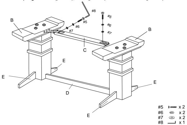
Step 4. Lay seat panel (part A) upside down on soft surface, such as carpet. Attach assembled unit (parts B, D & E) to seat panel (part A) using small flat washers (part #7), small spring washers (part #6), bolts (part #5) and allen wrench (part #8).
