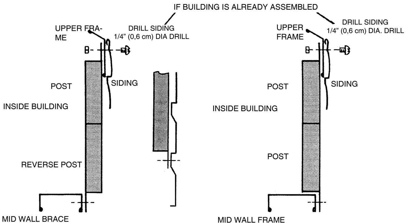
FOR BUILDINGS WITH NO MID WALL FRAME: Telescope posts to line up tab on bottom post with flat spot in siding panel. Fasten posts together with a bolt and nut. Using hole in bottom tab as a guide, drill 1/4" diameter hole through siding panel and fasten using a bolt and nut.
