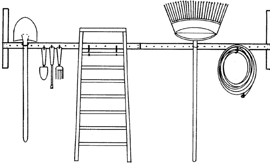
Kit can be attached through the sheet rock into studs or directly to studs using at least a #10 wood screw.
