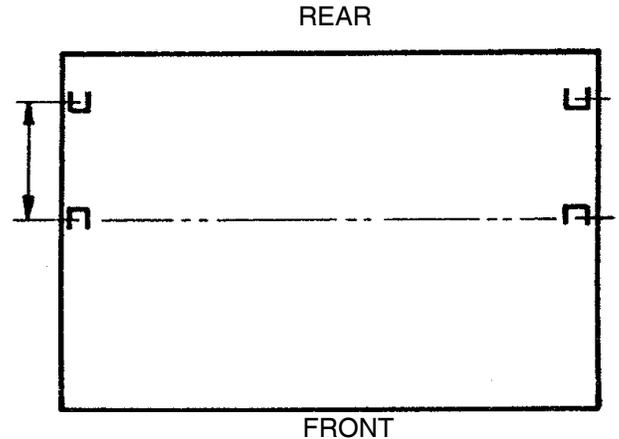
**2** Install the next two posts at either 26 3/8", 27 3/8" or 28 3/4" dimension (depending on your building) toward the front and remove the two fasteners as before. When complete, repeat procedure on the opposite side of building in the same manner.
