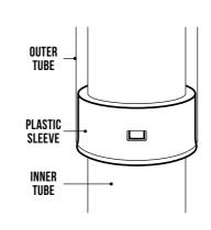
All side jacks come with a plastic sleeve fitting to prevent metal on metal grinding
