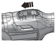
1. Push ON / OFF switch to turn ON.
