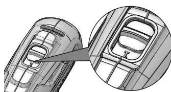
The machine has a two-speed switch designed for drilling or driving at LO (1) or HI (2) speeds. A slide switch is on top of the machine.
