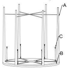
STEP.5 Tighten the bolt. (Tighten Bolts atter all bolts STEP. 6 Find product
