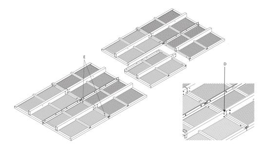
Step 3 | Assemble the 2 halves with 8 sets of M10x20mm bolts/nuts in area (F). Do not tighten hardware at this point.
