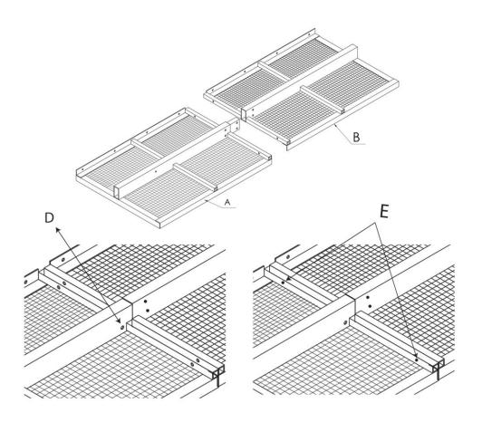
Step 2 Repeat same process with remaining sections. Do not tighten hardware at this point.
