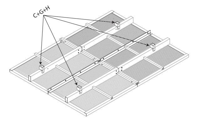
Step 5 To connect the assembled mesh deck to your utility cart frame (FTF-2200UW or ATV-2200HSH), attach the 4pcs frame connector parts (C) using the 4 sets of pre-assemble M8 x 65 (H) bolt/nut to the brackets located on the cart frame as shown in below illustration. Tighten all hardware when complete.
