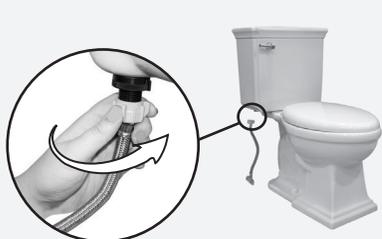
Note: We recommend replacing with a flexible supply line (pictured)
