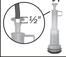
c) Attach other end of tube to refill adjuster. If tube kinks or is too long, trim prior to attaching.
