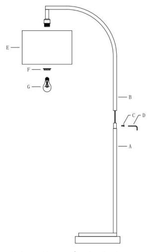
Step 1:Install the B part on the base with screw C and tooling D.
