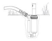
**DIG THE HOLE.** Dig the hole deep enough so the top of the sprinkler is level with the ground surface, about 9" deep and 4" across. IMPORTANT: make sure the unit is low enough to pass under your lawn mower.
