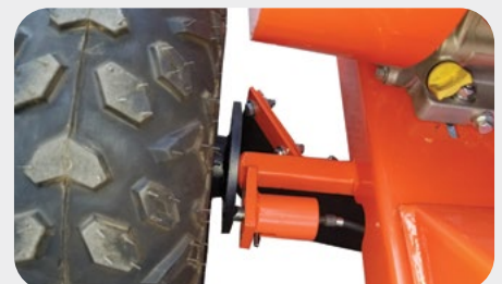
ATV wheels on HD axle. Tire 13.75D x 5.25W 145/70-6.
