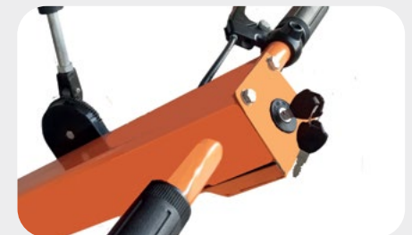
Lock out safety keys - Locking Throttle
