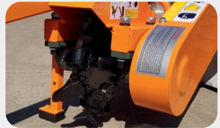
9 Carbide Cutting Head - Direct Drive
