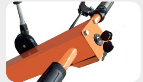
Lock out safety keys - Locking Throttle
