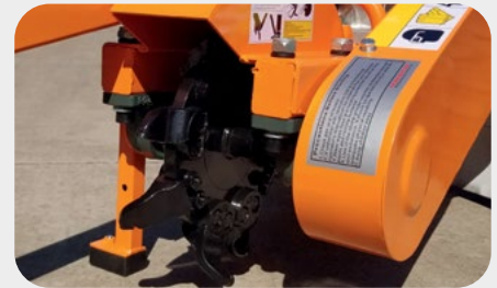
9 Carbide Cutting Head - Direct Drive
