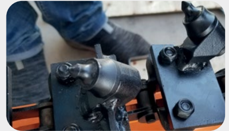
Tri-Cut High Carbide Teeth
