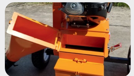
Extended Axle / Dual Swing Chutes / Tool Box
