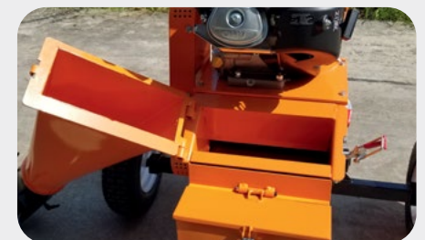
Extended Axle / Dual Swing Chutes / Tool Box
