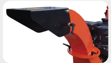
Rotational chip chute pickup truck bed height.
