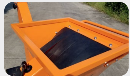
Large Feed Chute
