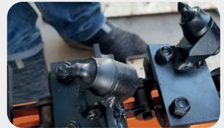
Tri-Cut High Carbide Teeth
