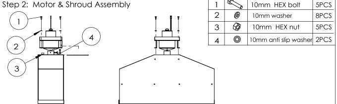
A. Align bolt holes on motor and shroud with bolt holes in the bottom of the hopper as shown. B. With the lid open. Insert bolts and washers from the outside as shown. Attach washers and 6mm hex nuts from the inside using a 10mm nut driver. Tighten firmly
