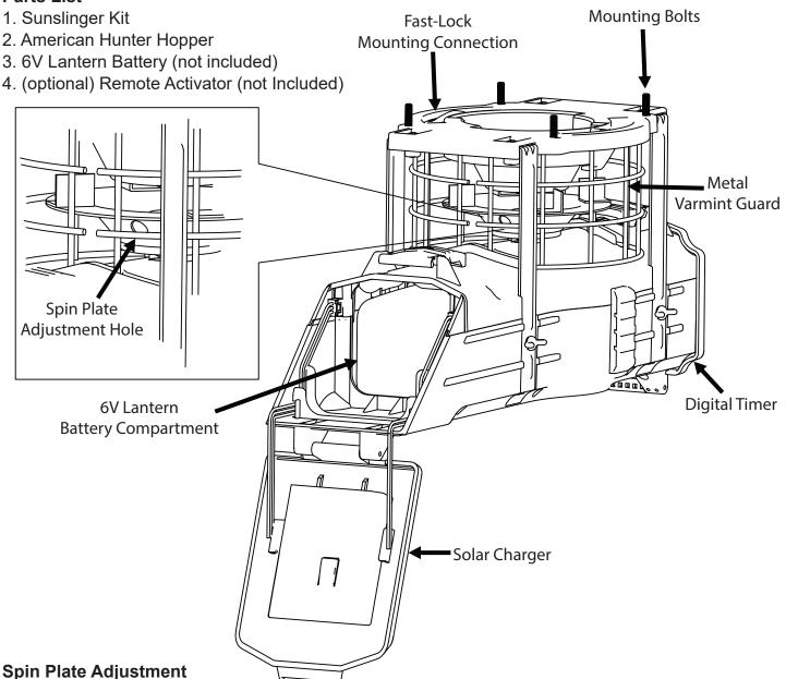
With the Sunslinger, you are able to raise and lower the spin plate to accomodate different feed sizes. NOTE: IT IS NOT NECESSARY TO REMOVE VARMINT GUARD TO ADJUST SPIN PLATE.
