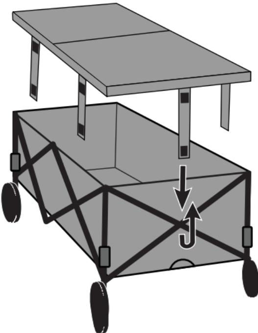
Guide table strap behind each cross point of the Adventure Wagon frame, then loop upward and fasten.
