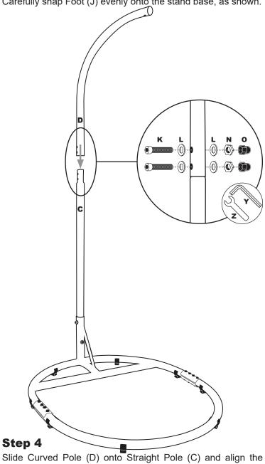
holes. Secure the poles using Bolt (K), Washer (L), and Lock Nut (N). Tighten the hardware using Large Hex Key (Y) and Spanner (Z). Place Large Hex Nut Cap (O) over the lock nut.
