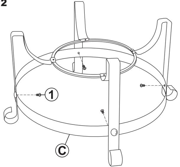
Align Large Ring (C) to the legs by hand-tightening three M6x8mm Bolts (1)
