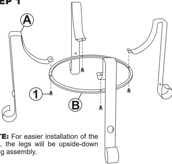
**NOTE:** For easier installation of the rings, the legs will be upside-down during assembly.
