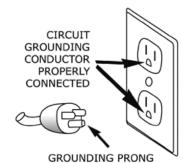
The unit should always be plugged into its own individual electrical outlet with a voltage rating that matches the rating label on the unit.
