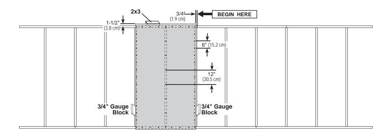
3 Install (5) **48**" **x 84**" panels flush to installed panels. Locate panels 1-1/2" from the top plate.
