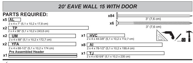
Orient parts on edge on floor as shown. Measure and mark from end of boards. Orient **Pre Assembled Header** as shown **(Fig. A)**. Secure with (2) 3" nails at each connection and (4) 3" nails at seams.
