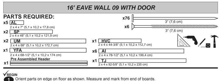
Orient **Pre Assembled Header** as shown (Fig. A).
