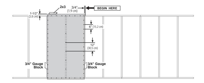
Install (4) 48" x 84" panels flush to installed panels. Locate panels 1-1/2" from the top plate.
