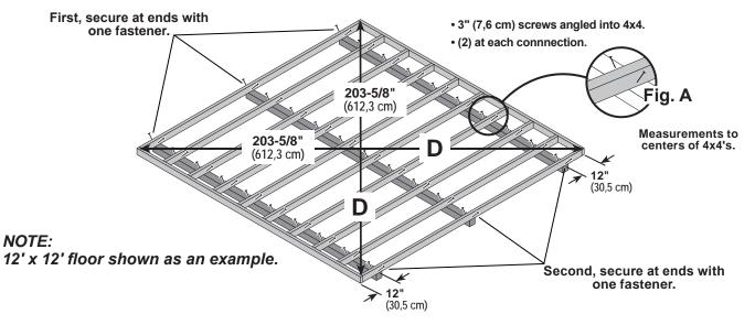
4x4 runners are generally installed 12" (30,5 cm) from ends of floor frame and under any seams.
