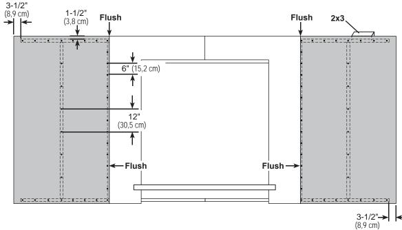
Your 16' eave wall 09 with door is now assembled. Carefully flip the wall over.
