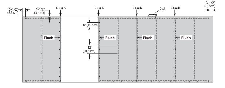
FINISH Your 20' eave wall 12 is now assembled. Carefully flip the wall over.
