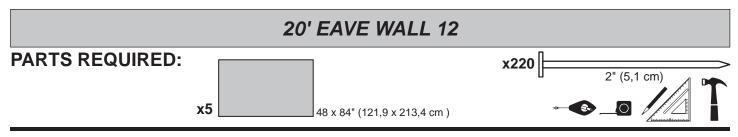
Install (1) 48" x 84" panel 1-1/2" from the top plate. Use a 2x3 spacer for consistent measurement.
