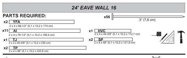
Orient parts on edge on floor. Measure and mark from end of boards. Secure with (2) 3" nails at each connection and (4) 3" nails at seams.
