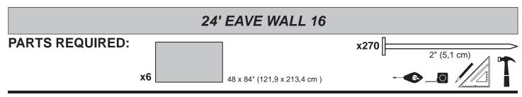
2 Install (1) 48" x 84" panel 1-1/2" from the top plate. Use a 2x3 spacer for consistent measurement.
