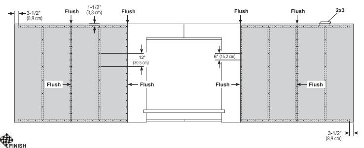
Your 24' eave wall 17 with door is now assembled. Carefully flip the wall over.
