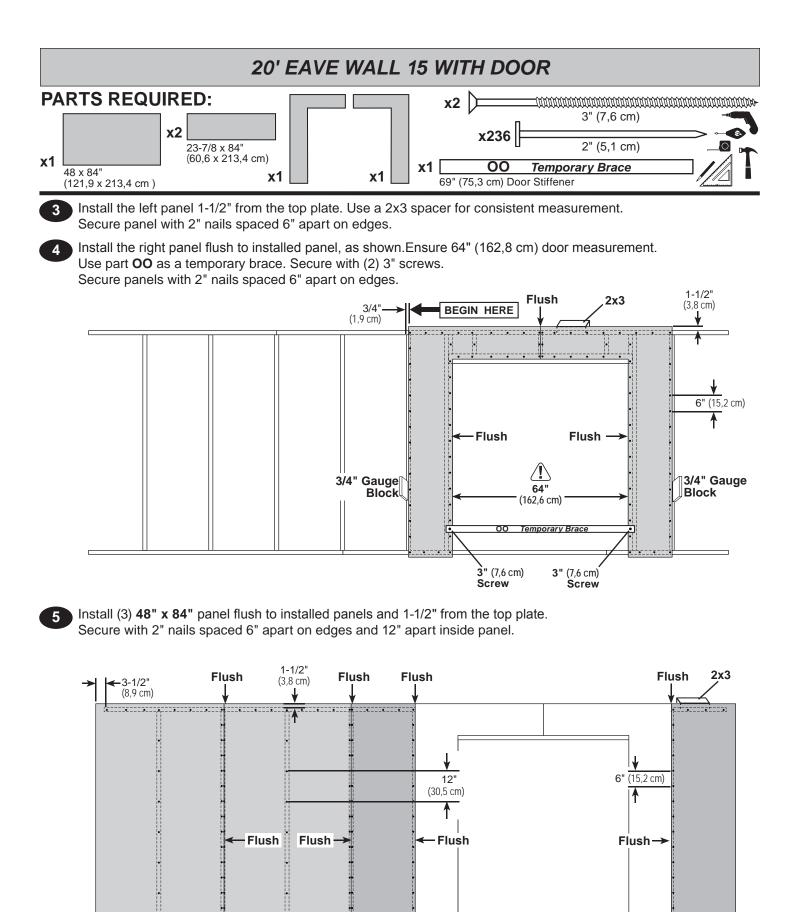
FINISH Your 20' eave wall 15 with door is now assembled. Carefully flip the wall over. 3-1/2". (8,9 cm)
