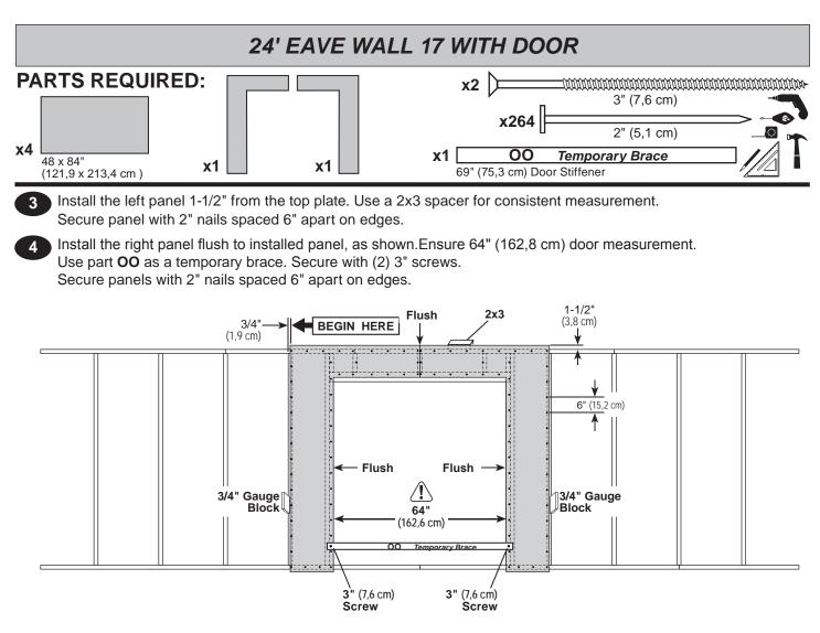
5 Install (2) **48" x 84"** panel flush to installed panels and 1-1/2" from the top plate. Secure with 2" nails spaced 6" apart on edges and 12" apart inside panel.
