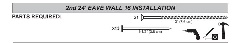
Secure 24' wall panel to 12' wall stud with 1-1/2" nails spaced 6" apart.
