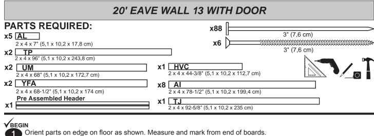
Orient parts on edge on floor as shown. Measure and mark from end of boards. Orient **Pre Assembled Header** as shown (**Fig. A**). Secure with (2) 3" nails at each connection and (4) 3" nails at seams.
