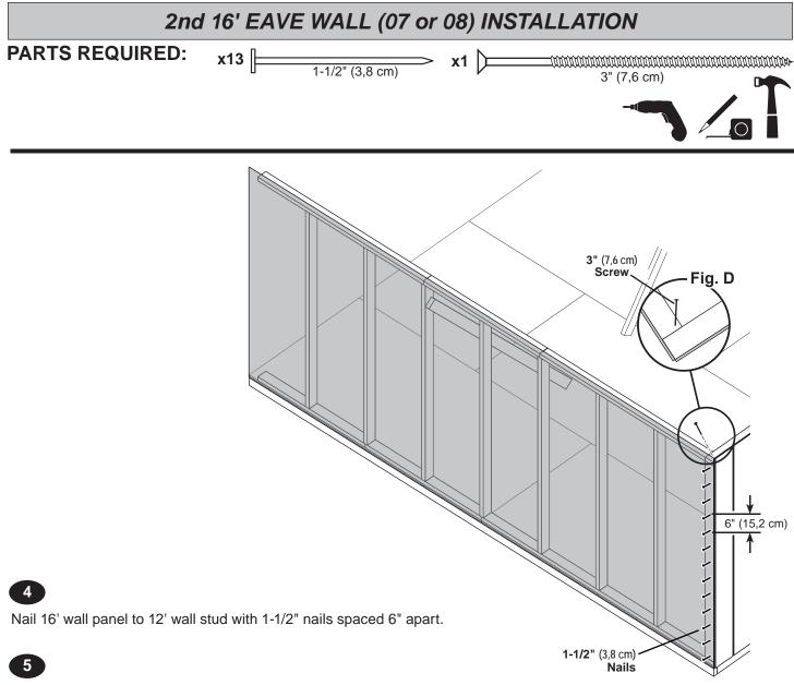
Secure gable wall top plate with (1) 3" screw at the corner at an angle, as shown (Fig. D).
