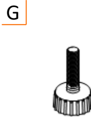
G FEET LEVELER (4) For stationary option
