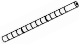
BOTTOM POLE (4) Threaded Insert (4) pre-installed
