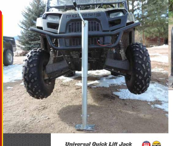
The Hornet Outdoors Universal Quick Lift Jack was designed for off-road ATV/UTV use and also makes a great jack for your snowmobile or ATV/UTV trailer. It is lightweight, has a high capacity and long extension range, and is simple to use. Operate with the included crank handle, or remove the handle and use a ratchet or cordless drill. It will easily lift your ATV, UTV, trailer, or other small vehicle. Two Models available are:
